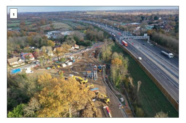
Figure 2-3 - Aerial view of construction of new southern roundabout
